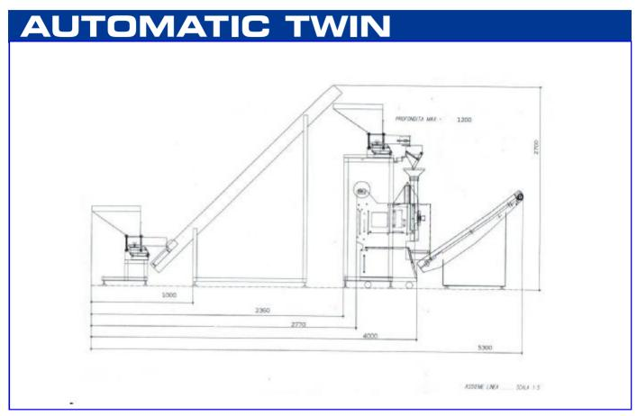
Vertical form, fill and seal packaging machine with incredible working possibilities represented by quality and reliability.
